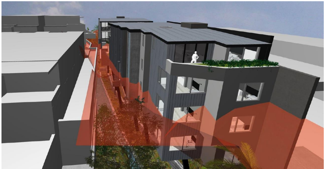
Figure 2 - Contextual height blanket diagram showing the relationship of the proposed building to the height established by the adjoining properties
