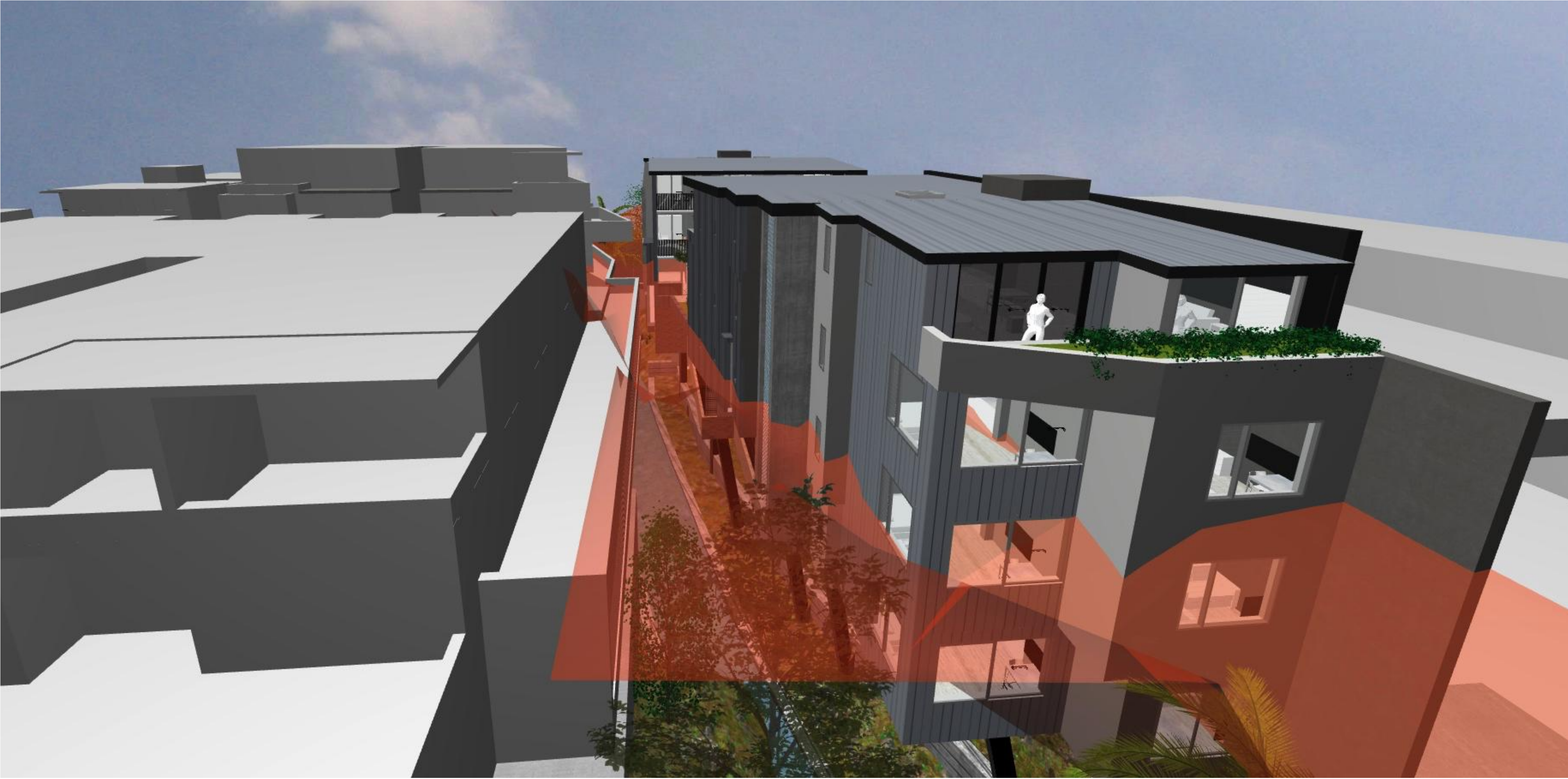
11M HEIGHT PLANE ABOVE GROUND LEVEL (EXISTING)
